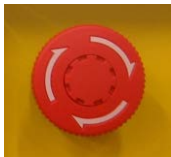
Fig. 14 Emergency stop button
