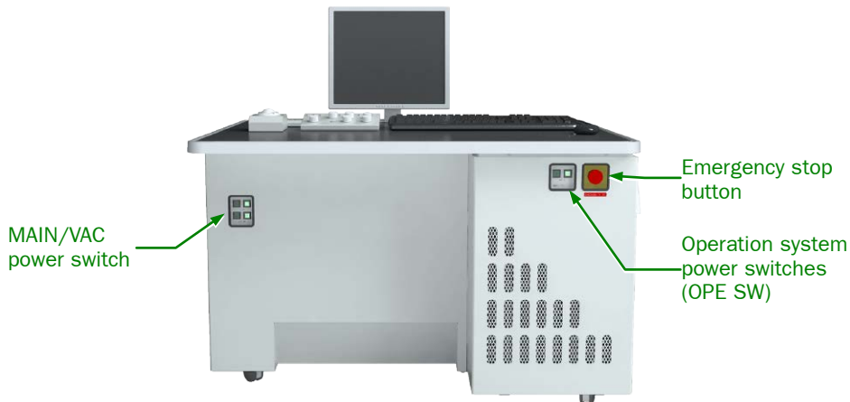
Fig. 11 Front of the operation console
