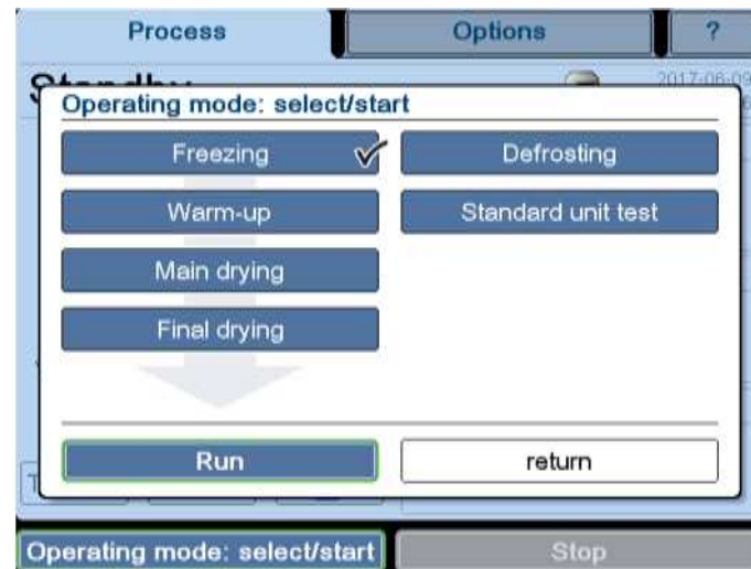
Fig. 27: Dialogue box "Operating mode: select/start" (The version of the dialogue box that is displayed depends on the equipment of the freeze-dryer.)
