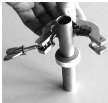
Fig. 53: Attaching the clamping ring
