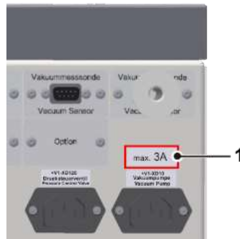
Fig. 13: Indication of the maximum current for the vacuum pump (example)
