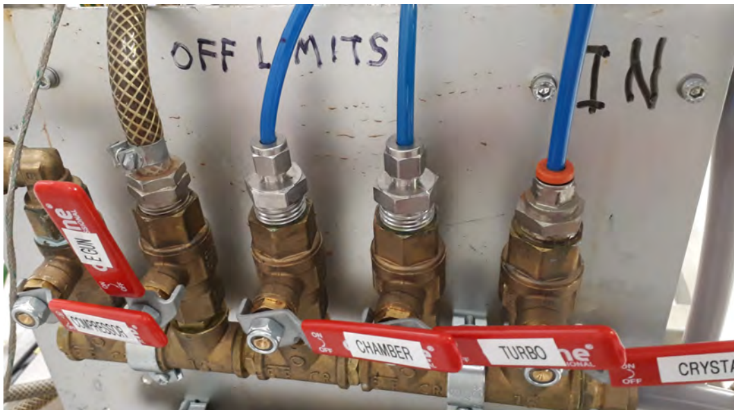
Figure 4: Correct positions for the water valves. Evaporator should be fully open, others only partially.
