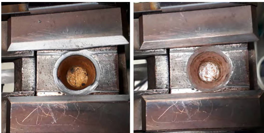
Figure 3: Left: Pocket with material accumulation. Right: Cleaned pocket.
