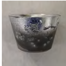
Figure 2: A crucible where the material has spilled over and needs to be replaced.
