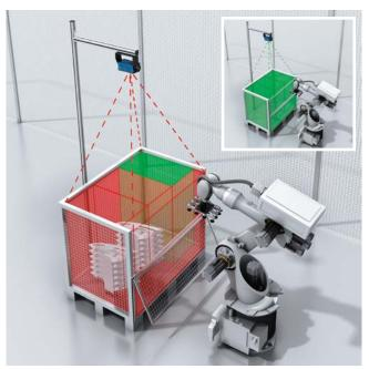
The Visionary-T DT installed vertically above the storage container reliably detects that the container is in the correct position and that the door is closed. It also reports whether there are any objects in the container and, if so, where. It therefore provides the robot with valuable information and prevents errors such as overloading.
