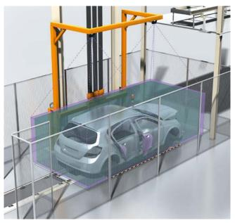
By recognizing any changes in the detection volume, for example due to open doors, the Visionary-T DT helps avoid damage during lifting processes in automotive manufacturing.
