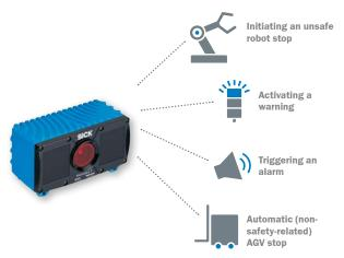
The Visionary-T DT evaluates the received 3D data directly without computer support, and delivers four digital output signals that can be used to initiate a variety of actions. This illustration shows four examples.
