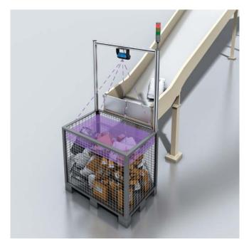
The Visionary-T DT recognizes immediately that a storage container has been filled to a predefined level. Before overflow can occur, the sensor issues a timely visual or acoustic warning resulting in an appropriate machine response (e.g., closing of the slide).
