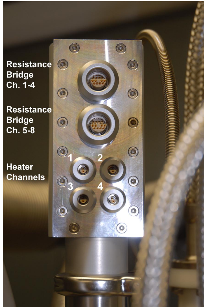
Figure 15. DR wiring connector box.
