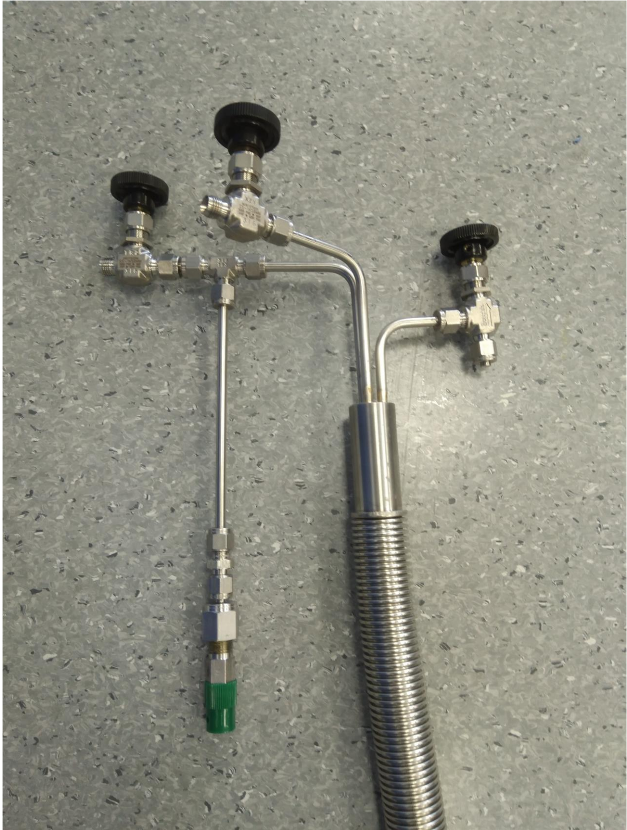
Figure 2. The shortest line with a Swagelok blind is used to maintain vacuum inside the transfer line (the black knob is removed). Input and output sides are labelled, the line with the overpressure relief valve (green cap) is the output side. All connections are 6 mm Swagelok.
