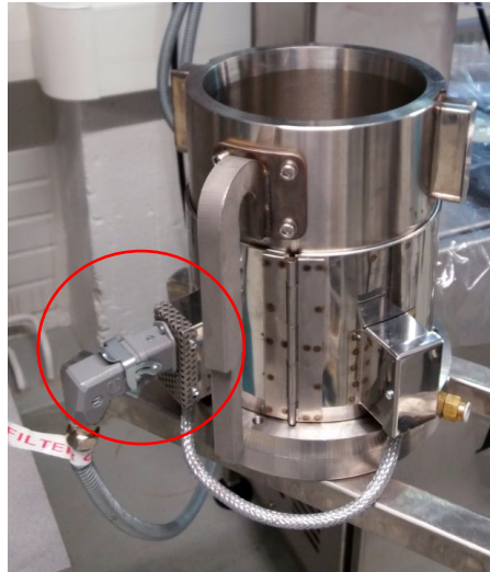
Figure 8 – Heating up the filtration unit
