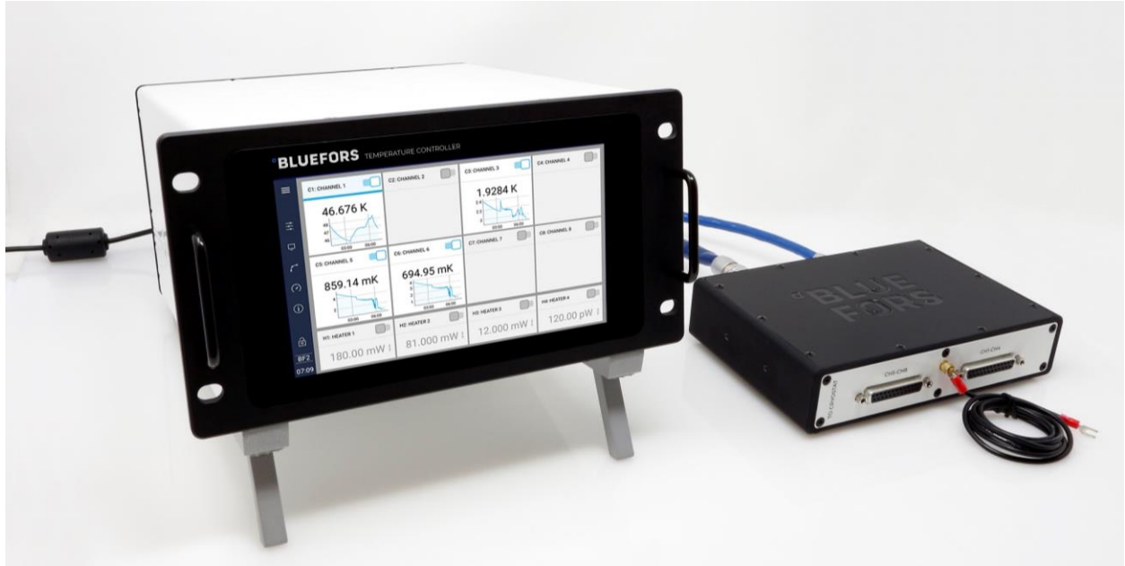
Figure 1: Control Unit and Pre-Amplifier
