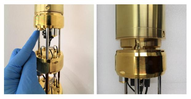
The sample space of the probe and the DC wiring is thermally isolated from the hotter stages with a detach mechanism. The detach mechanism is unlocked by pressing the key pin shown in picture above. This should always be done before inserting the probe to the cryostat.
