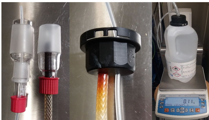
Figure 4 - Acid bottle with the special cap and its connectors
