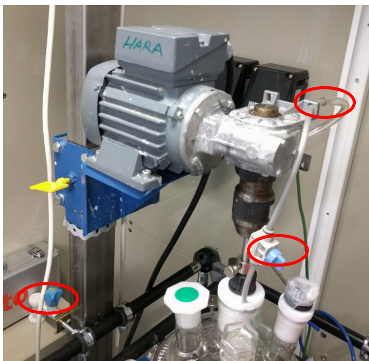
Figure 11 - Drying the reactor with compressed air
