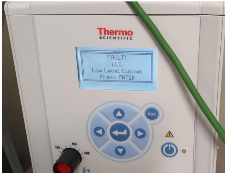
Figure 14 – Thermostat low water level -error
