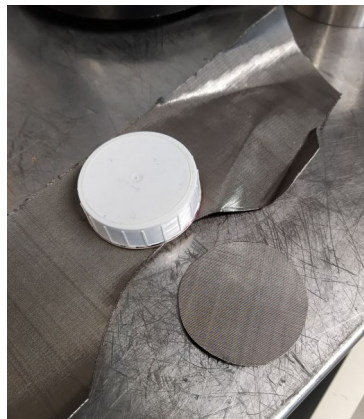
Image 2 - Cutting template for filter (Small cylinder)
