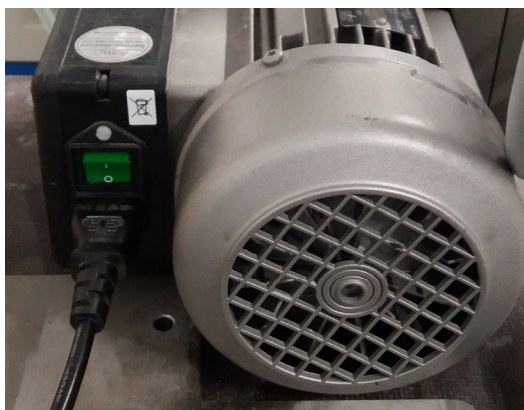
Image 4 - Vacuum pump power switch
