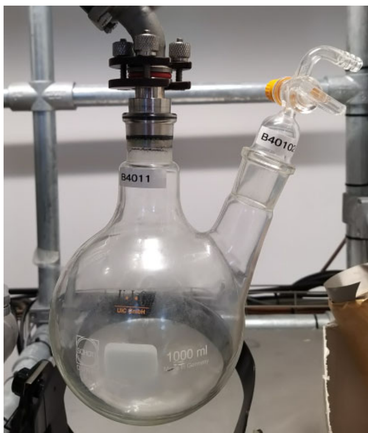
Image 10 - Liquid Trap Discharge Flask
