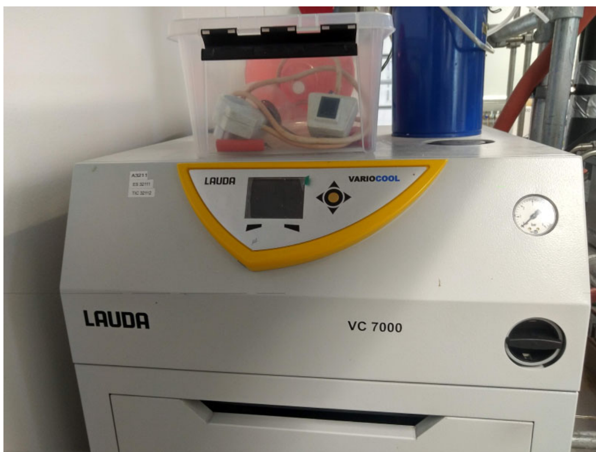
Image 7 - Cooling unit for the Condenser
