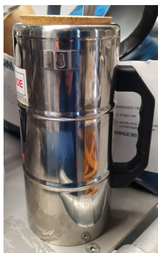
Image 3 - A Dewar for pouring Liquid Nitrogen
