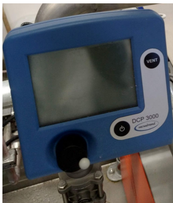
Image 11 - Pressure gauge control panel
