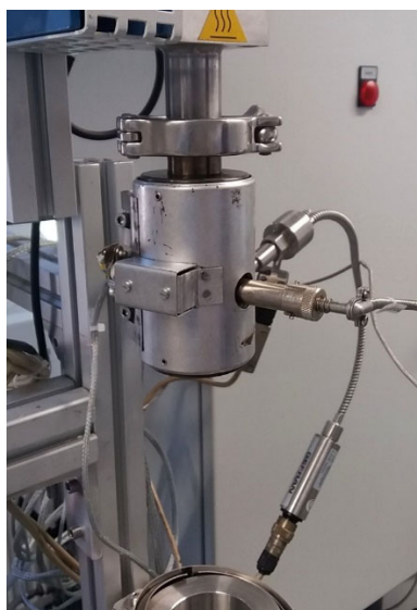
Image 9 - Cylinder unit assembled, and sensors attached
