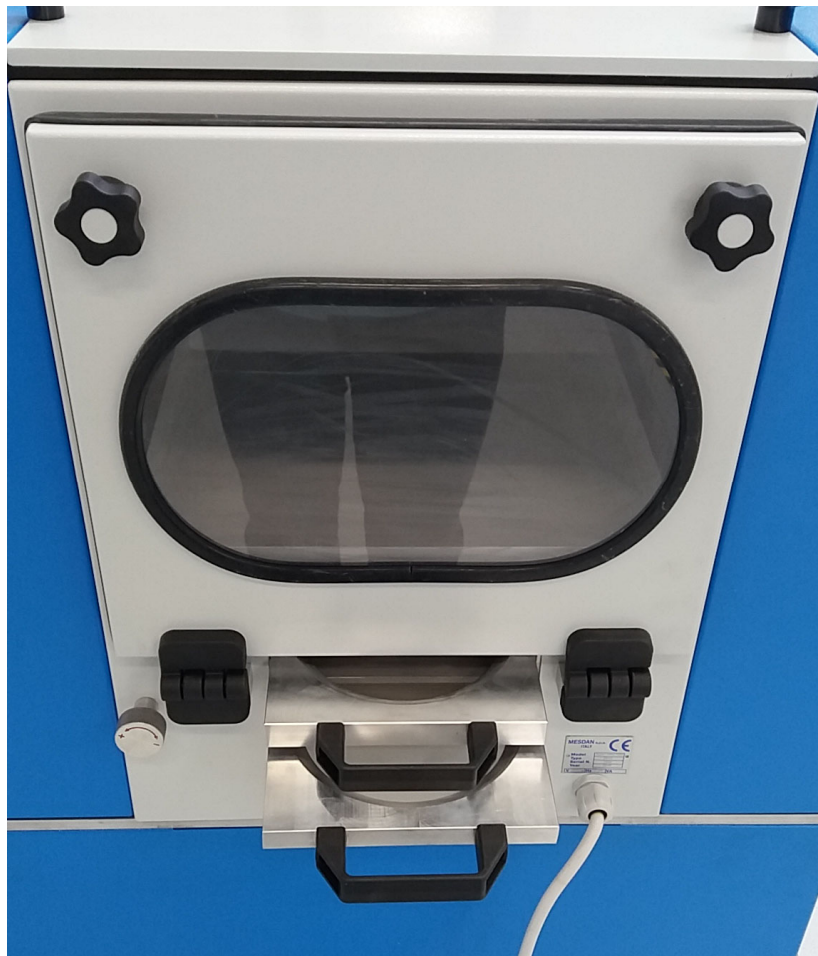
Image 2 – Collector compartment and filters
