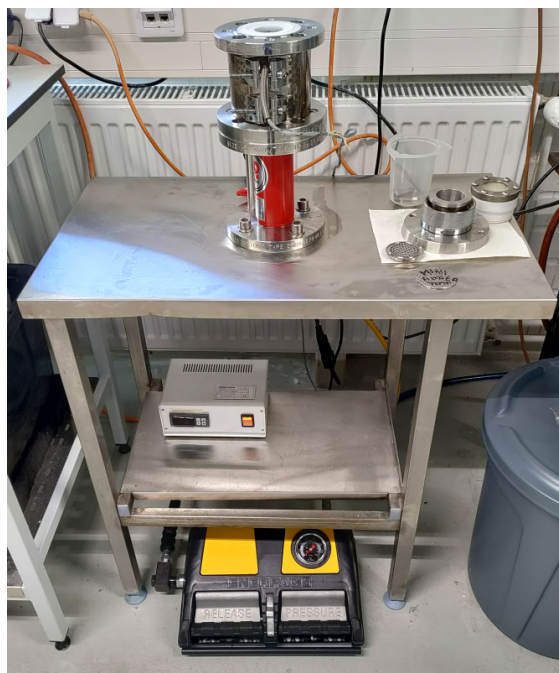
Image 1 – Filtration unit without safety hood
