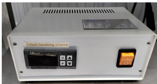
Image 4 – Heating controller unit
