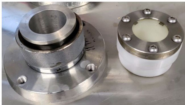
Image 5 – Filtrate cylinder safety cover installation
