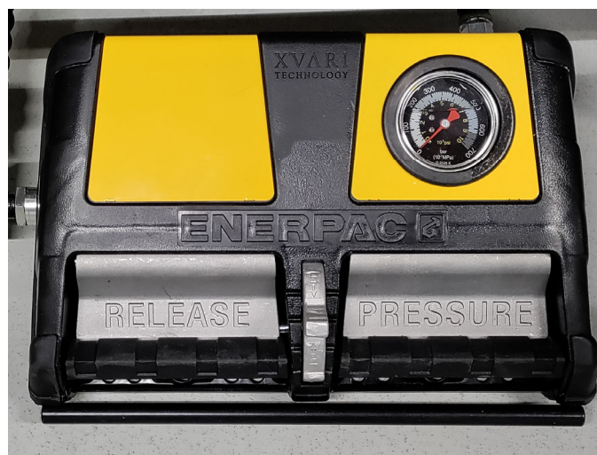
Image 7 – Piston control unit (Enerpac XA11G)
